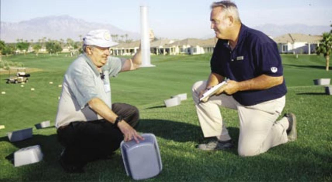
**Checking sprinkler efficiency**—From left, Don Ackley, water management supervisor, and Robert White, golf course superintendent at Heritage Palms, measure water samples collected in a sprinkler test to determine if water is being evenly applied.
