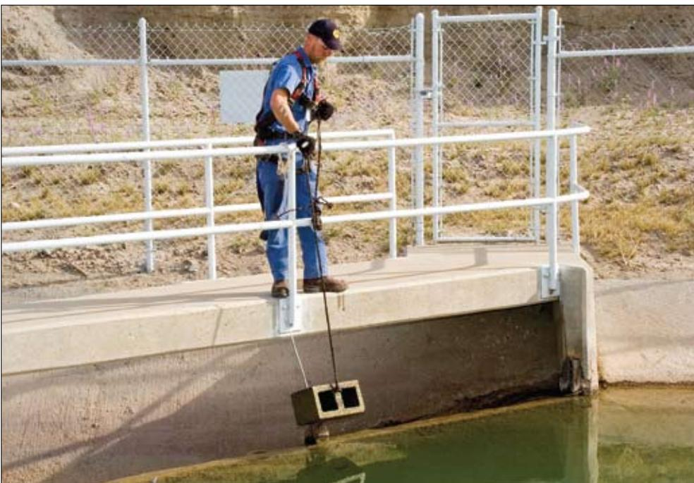
Quagga mussels will attach to anything in which they come in contact, including canals, pipes and water treatment facilities. They haven't entered the Coachella Canal system yet, but employees are monitoring for their existence using cinder blocks, placed at six different stations along the stretch of the 122-mile canal.
